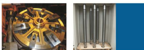
刻划机高精度机械零件——大尺度、高精度涡轮，高精度丝杠 High precision parts of ruling engine—large scale wheel and lead screw with high precision
