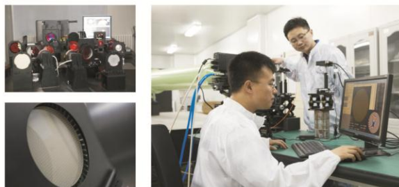
961单元压电变形反射镜及自适应光学系统 961-element piezoelectric deformable mirror and adaptive optics systems
