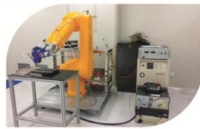
半导体激光焊接光源 High-Power Diode Laser for Laser Welding
